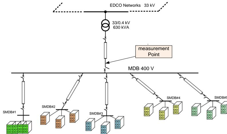
Fig. 1. Single line diagram for the system under the study
