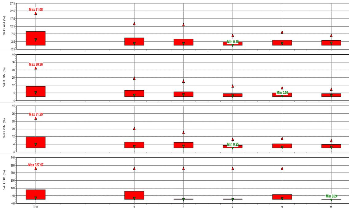
Fig. 6. Harmonics Spectrum and THD for phase currents: red triangle: maximum value; green triangle: minimum value; red bar: average value
