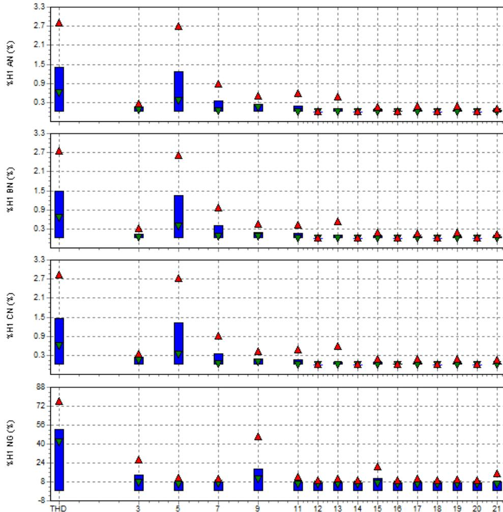
Fig. 3. Harmonics spectrum and THD for phase voltages: (red triangle: maximum value; green triangle: minimum value; blue bar: average value)
